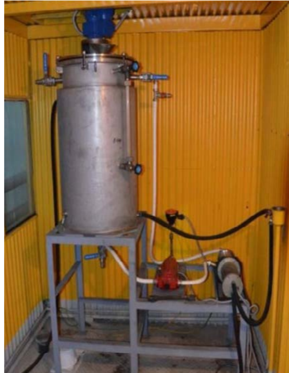
Pilot device to obtain additives. Capacity 450 ...500 l/shift (for 5000 tons of gasoline)
