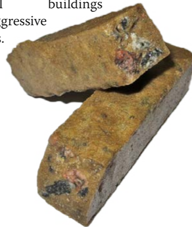
Polymer concrete samples after flexural strength test
