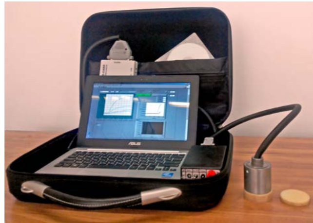
Portable device for nondestructive control of thermal material properties and time/temperature properties of structural transformations in polymeric materials.
