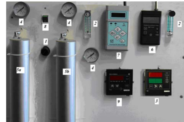
Lab stand of oxygen-enriched air production system: 1 – control valve; 2 – rotameter; 3 – multichannel flow meter; 4 – manometer; 5 a, b – absorbers; 6 – moisture-in-gas meter; 7 – oxygen concentration meter; 8 – switch button; 9 – time relay.
