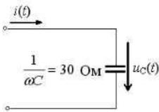
:-  $i(t) = 5\sin(100t + 60^\circ) + 1\sin(200t + 30^\circ)$ ;    -:  $i(t) = 5\sin(100t + 150^\circ) + 1\sin(200t + 120^\circ)$ ;
