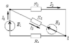
$$\therefore I_1 - I_2 - I_3 = 0; \quad \therefore I_1 - I_2 + I_3 = 0; \quad \therefore -I_1 - I_2 + I_3 = 0; \quad \therefore I_1 + I_2 + I_3 = 0.$$
