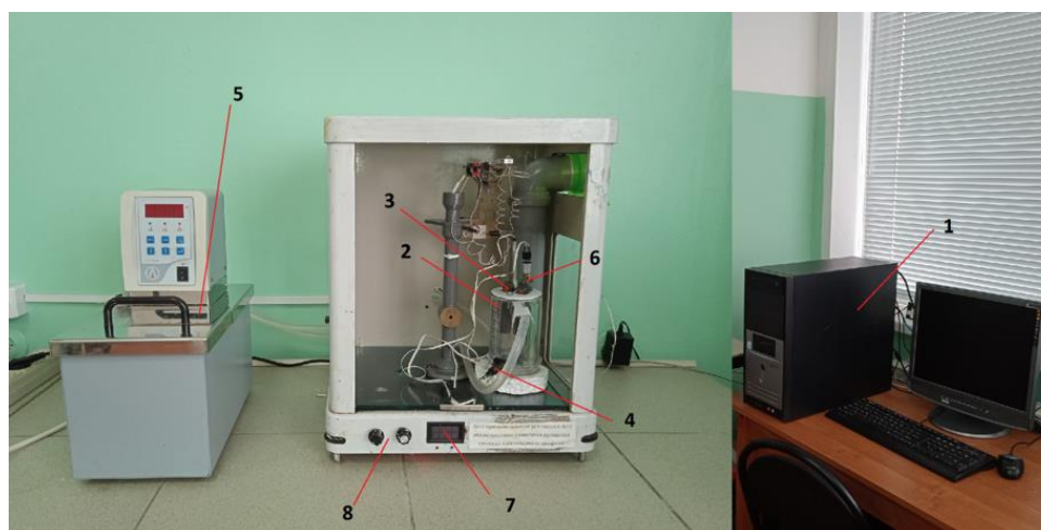
Figure 1 - Installation for studying the kinetics of electrochemical synthesis of colloidal graphite 1 - personal computer; 2 - electrochemical cell; 3 - current-carrying clamps; 4 - optical sensor; 5 - liquid thermostat; 6 - agitator. 7 - measuring instrument screen, 8 - variable resistor adjustment knobs.
