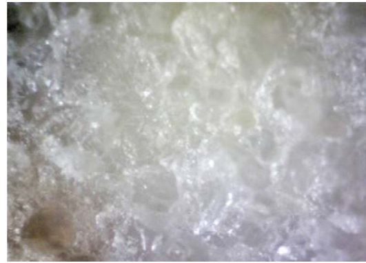
Microstructure of polymer concrete containing 6% broken glass, 64-power magnification
