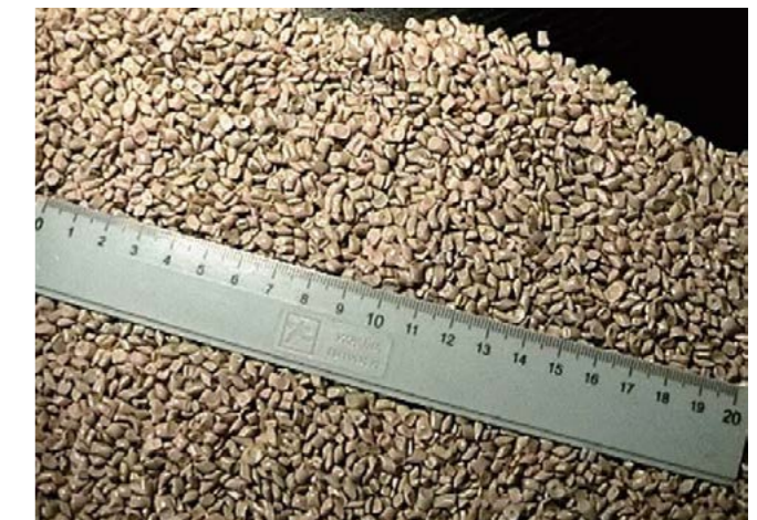
Recycled granulated material produced by roller-screw assembly
