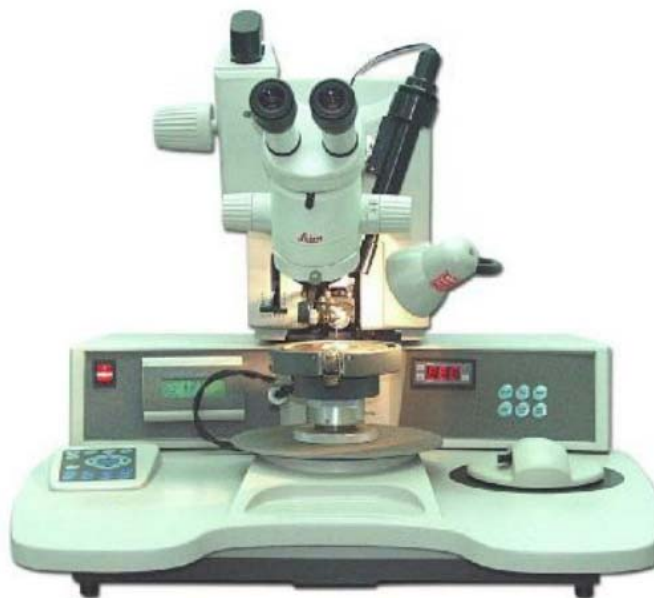
Fig. 2 - Installation for ultrasonic welding of the microwire connections of Kulicke&Soffa 4700AD company
